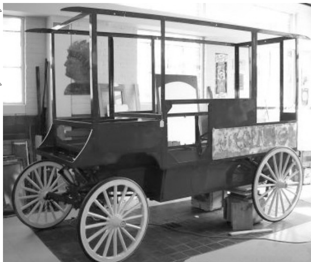
This 1914 Cretors popcorn wagon is partway through its restoration at the Brown County Historical Society using a combination of original and replacement parts. For safety reasons, it will be restored without gas burners. When completed, the wagon will be used at community events.
