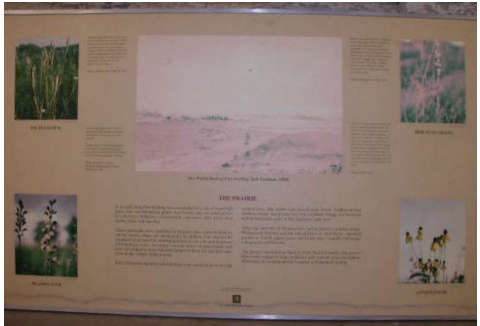
This fiberglass panel shows fading from exposure to ultraviolet light. Though they have a relatively short lifespan, fiberglass panels are inexpensive to produce so multiples can be ordered for replacement as needed.
