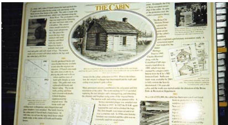
Porcelain enamel panels are durable and stable but expensive to produce.
